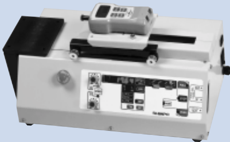
FGE with FGS-50PXH horizontal motorized test stand
