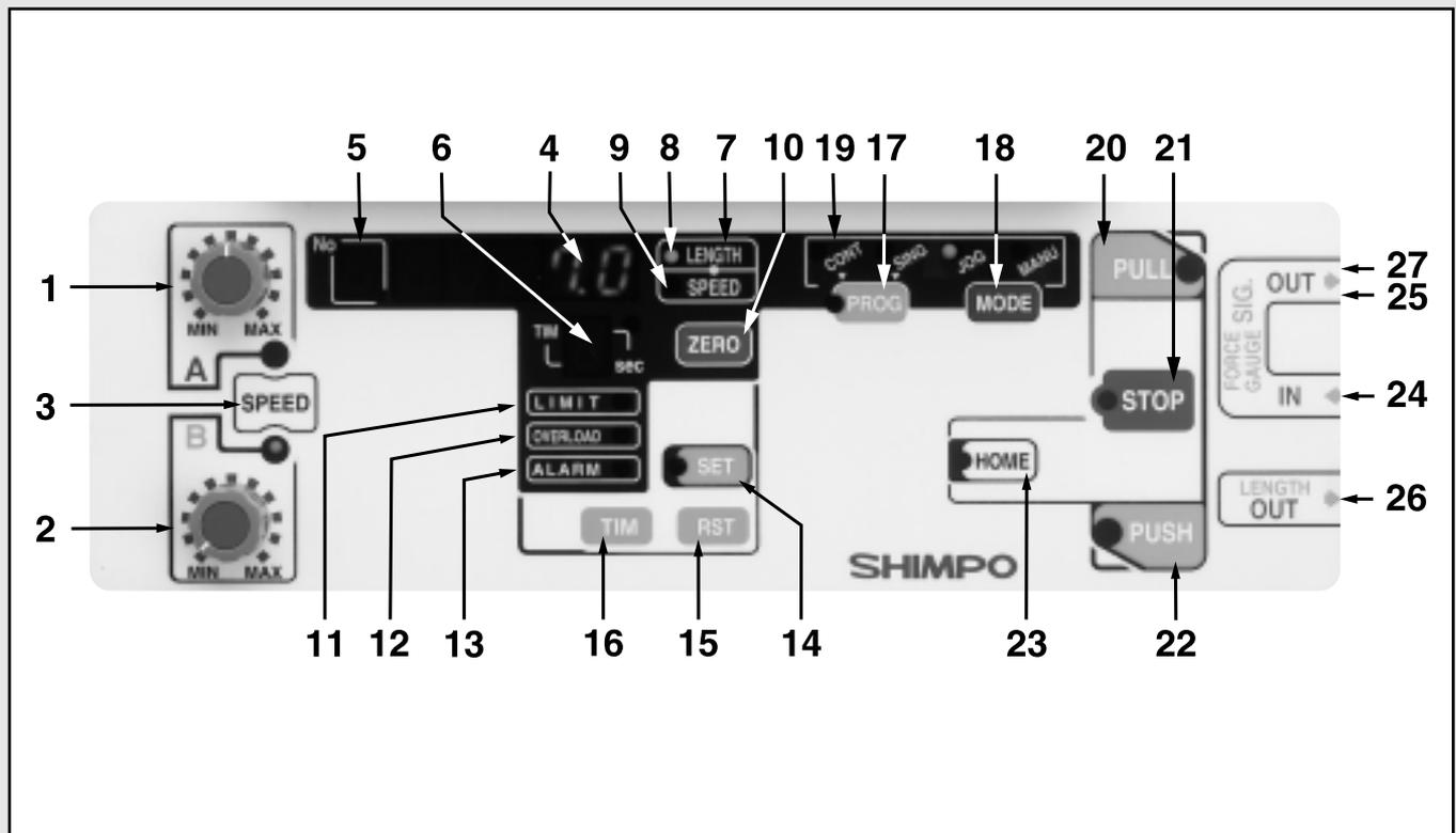
1. **Speed A control knob:** Changes the A speed of the force gauge plate
