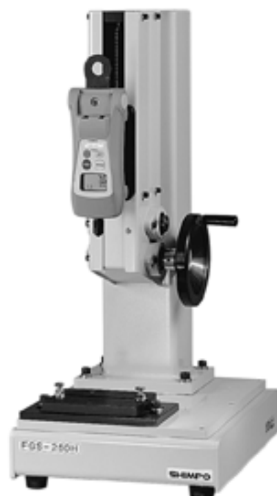
FGS-250H manual test stand (shown with FGE-H)
