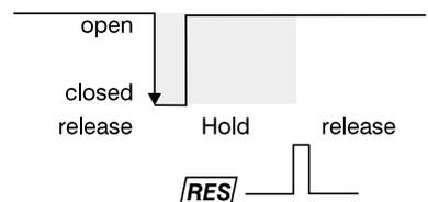
HOLD cannot be released from an external source in the edge trigger mode. To release it press RESET. Level mode can be released externally.
