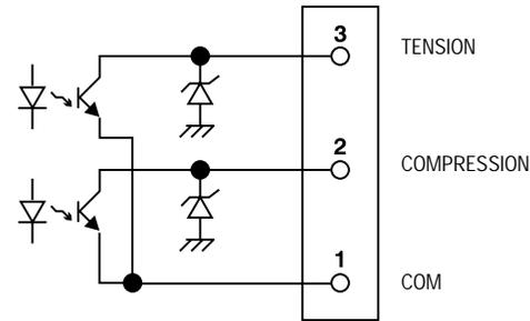
Both transistors can handle up to 28VDC, 5 mA.
