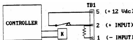
**Figure 3-4. On/Off control (Output Enabled by Contact Closure)**
