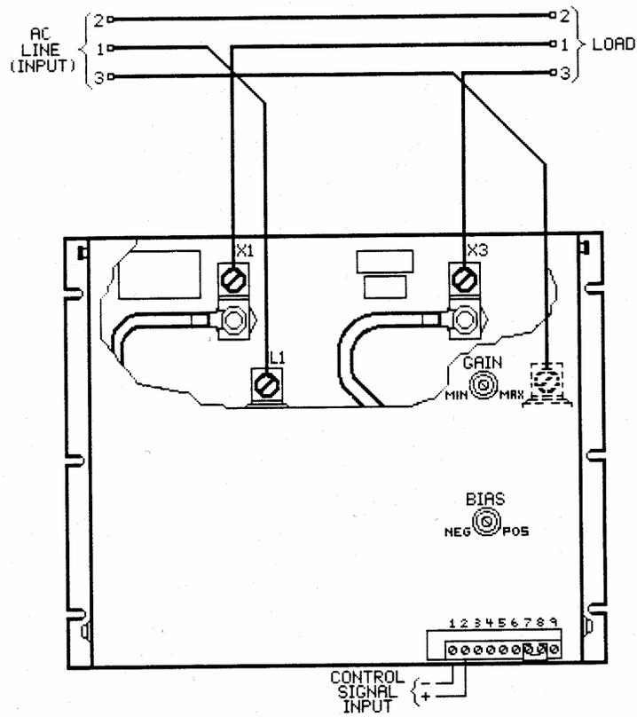
Figure 2-1. Typical 2Z Line and Load Connections
