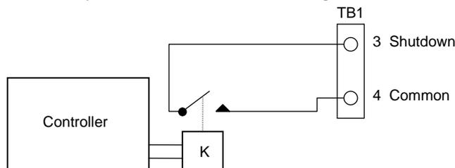
Figure 2-7. Shutdown (Output Disabled by Contact Closure)
