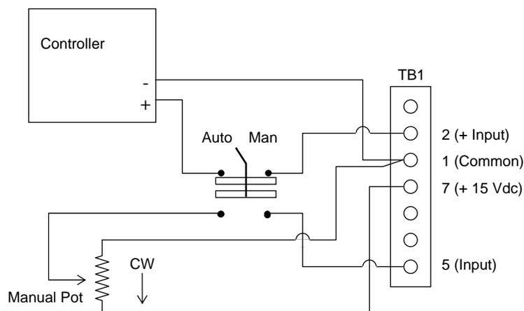
Figure 2-6. Auto/Manual Control with Controller and Remote Potentiometer
