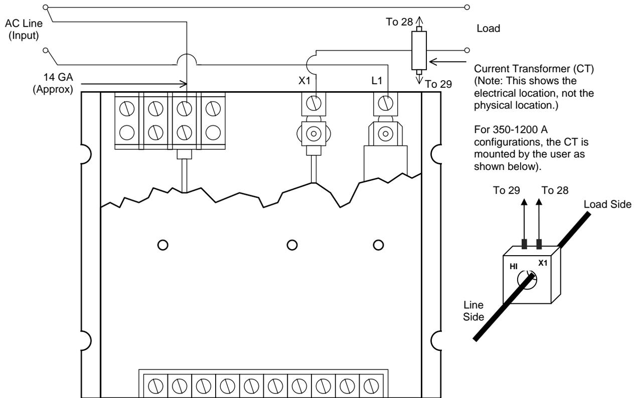
Figure 2-3. Typical 1PCI Line and Load Connections
