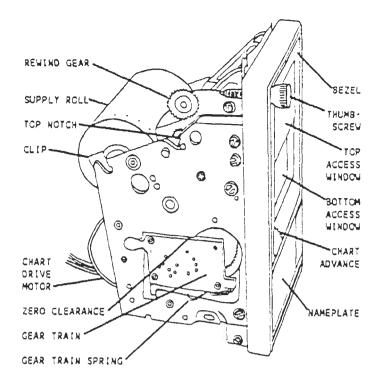
Figure 2 Basic Chart Drive With Case Removed
