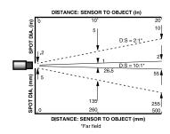
D:S is the optical resolution expressed as a ratio of the distance to the resolution spot divided by the diameter of the spot. Optical resolution for the MI is 2:1 and 10:1.
