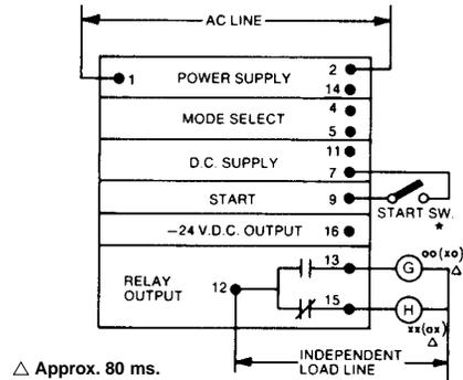
\*Start switch must be closed — or DC start signal must be **on** — for entire cycle. Timer resets when start switch opens or DC start signal turns **off**. to start from DC voltage, apply external ground on 11 and start signal on 9.
