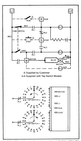
**CAUTION:** When command output signal is applied to either the Step or Run terminal, an output appears on the other terminal. In the case of a signal on the Step terminal, the output signal is momentary. A command input signal on the run terminal, the output signal on the step terminal appears until command signal is removed.
